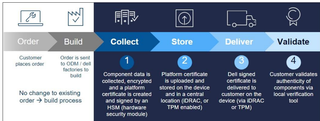
図3. Dell Secured Component Verification (SCV)
